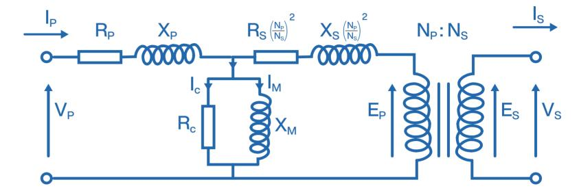
Winding joule losses and leakage reactances are approximated by loop impedances  $R_{p}$ ,  $R_{s}$  and  $X_{p}$ ,  $X_{s}$ . Core losses:  $R_{c}$  and  $X_{M}$  (magnetizing reactance).
